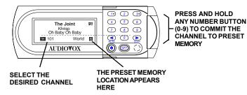
Figure 10. Setting Preset Channels
